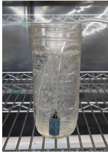
Left: aerated water setup with an aquarium bubbler. Right: still water setup.
