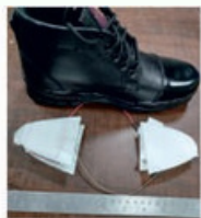
Position of TENG inside the sole
