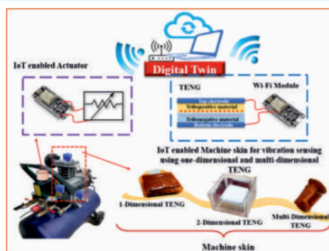
Schematic of the Machine skin and actuator on the air compressor incorporated with its Digital Twin
