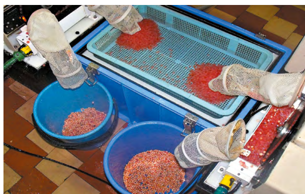
Fig. 9.17. Egg sorting using egg-sorting machines. Dead eggs are in buckets; live eggs, bright red in colour can be seen on the mesh tray
