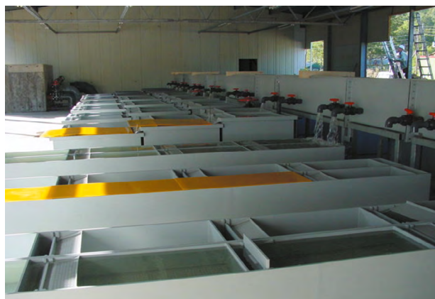
Fig. 9.16. Atkins-type incubators in the hatchery incubation department
