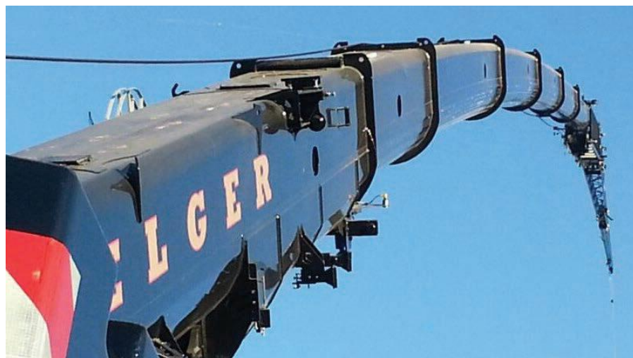
Fig. 3. Hydraulic boom section bend when loaded increases the radius, requiring booming up to prevent overloading.
