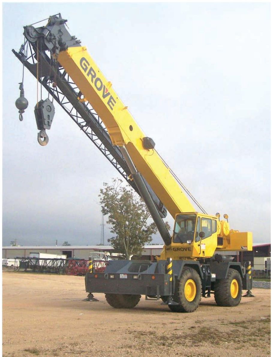
Fig. 1. The versatile self-propelled hydraulic crane, Grove RT540 E.
