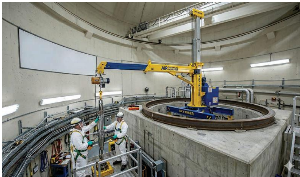
The SKY RISER, a custom-engineered, compact nuclear reactor crane, was designed by Air Technical Industries (ATI) specifically to mount on the rim of the reactor.
