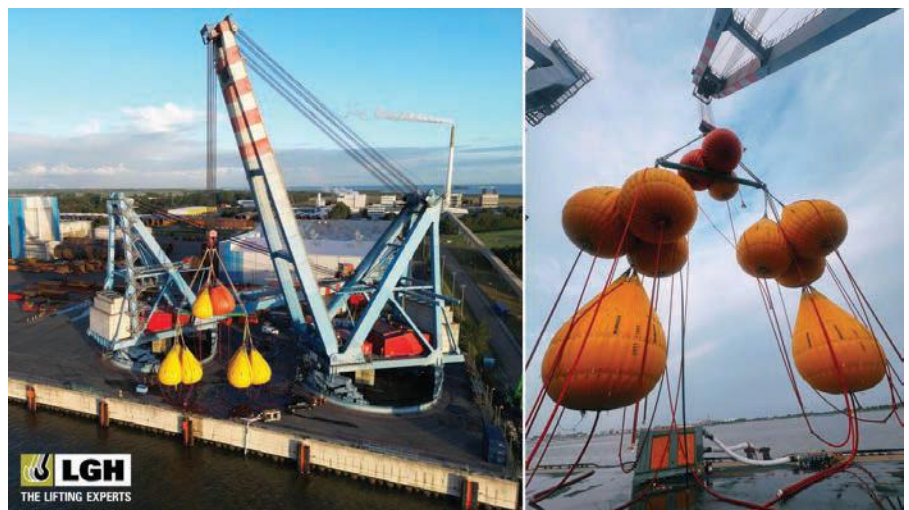
Modulift Spreader Beam conducting load test in Weser, Germany.
