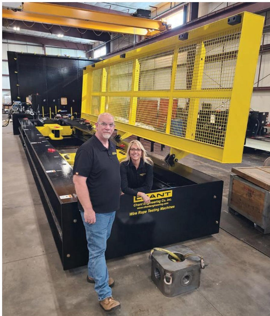
John Organsky (left), Technical Sales Representative, and Sharon Mathis (right), Chant Engineering Sales Manager, stand in front of a 1.3 million lb. (600 MT) horizontal proof test machine at Chant Engineering’s New Britain, Pennsylvania facility.
