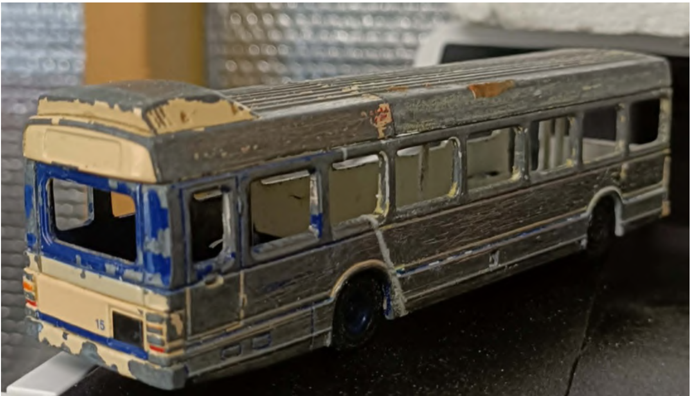
The British Airways Leyland National needed a significant amount of chopping so another damaged EFE was used. Cuts were made to remove half of the front and all of the front entrance and to accommodate an extra set of doors on the offside.
