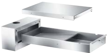
APCL 021 Lint filter box, stainless steel, removes lint and coarser particles from wash liquor. • For installation on a suitable plinth • Removable for quick and easy cleaning. • Easily removable fluff filter in stainless steel • Volume 24 l • Diameter of rear connector 70 mm • H/W/D: 25.00 cm - 49.85 cm - 86.00 cm
