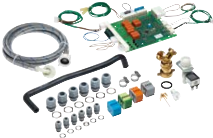
APWM 077 MF-01 24/32 multi-function module, for additional machine functions. • Suitable for PW 6241, PW 6321 • For controlling dispensing pumps 1-6, incl. empty sensing • For controlling an external signal at programme stop • For connection to an energy management system • For stopping the programme from outside
