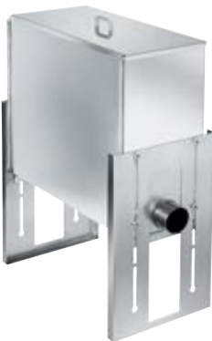
APWM 900 Lint filter box made from stainless steel to remove lint and coarser particles from wash liquor. • For use with heavily soiled fabrics • Volume approx. 70 l, adjustable installation height 0–250 mm • For connection to washing machines on a plinth • Easily removable fluff filter in stainless steel • Ø connection: 7.5 cm • H/W/D: 54.30 cm - 31.00 cm - 64.80 cm
