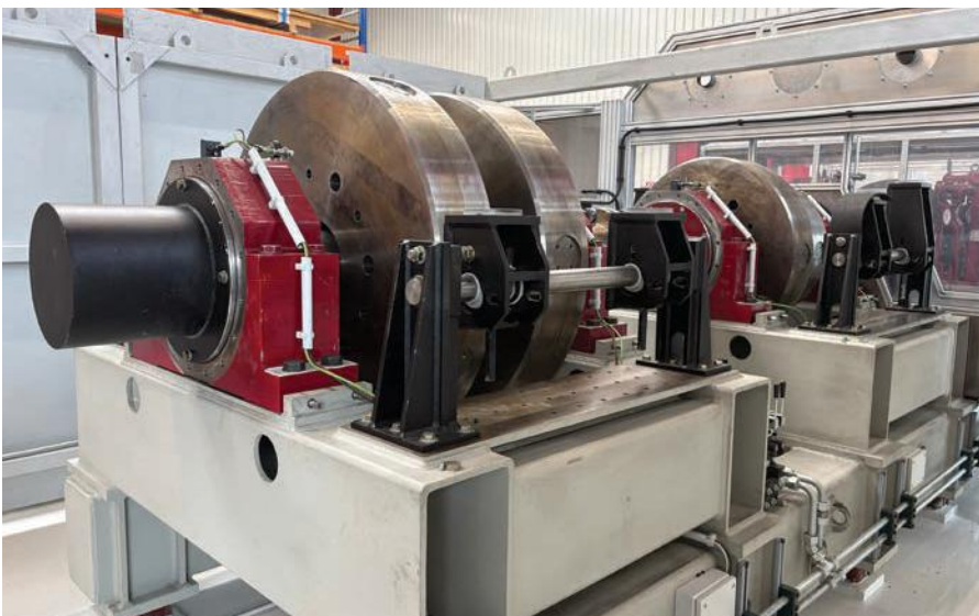
Fly wheel mass section of large dyno test bench at Dellner Bubenzer.
