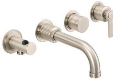
4 Hole Concealed Bath Mixer with Diverter without Hand Shower without Hose Spout Length 196 mm Min. Operating Pressure 1.5 bar MP
