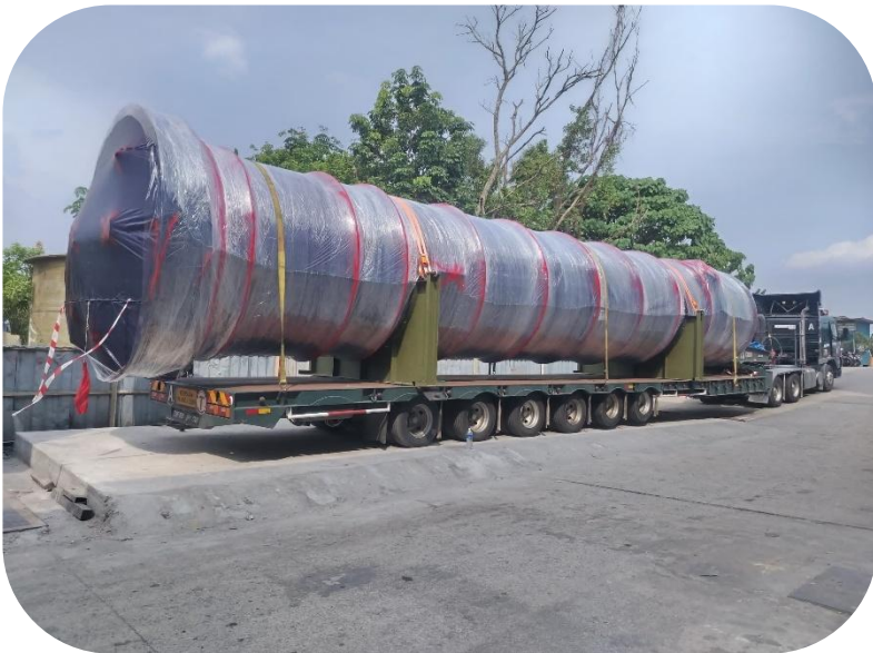
Ion exchange columns being transported to site
