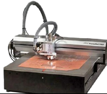
CNC MILLING MACHINE FOR DOUBLE LAYER PCB PROTOTYPING (LPKF ROUTER SYSTEM)
