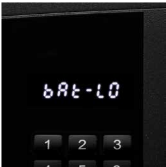
Low battery indicator Standard models displays "LO-BAT," while the Premium model shows "BAT-LO" on its screen
