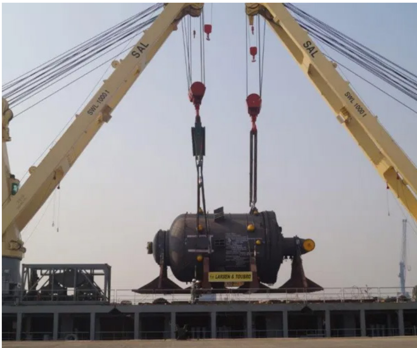
M.V. Lone loaded 1 Unit Ethylene Oxide Reactor 1324 metric tons (Weight along with lifting gear) Dimensions – 21.300 X 13.00 X 10.250 meters ( L X B X H ) in 2013
