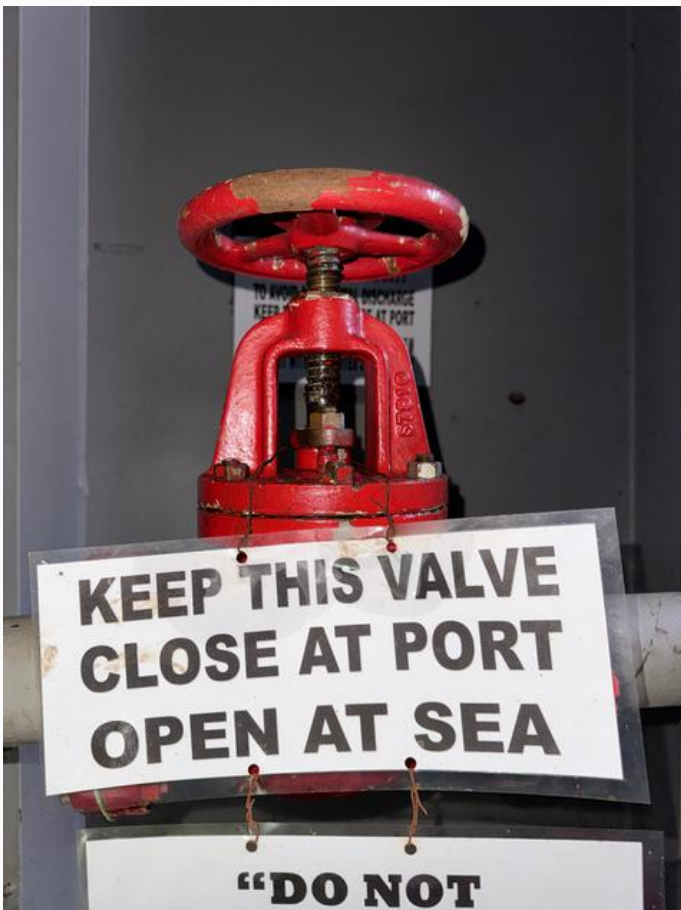
2. During a routine deck inspection, a forward dewatering valve was found in the open position while the vessel was alongside. The operating instruction attached to the valve clearly stated: KEEP THIS VALVE CLOSED AT PORT – OPEN AT SEA
