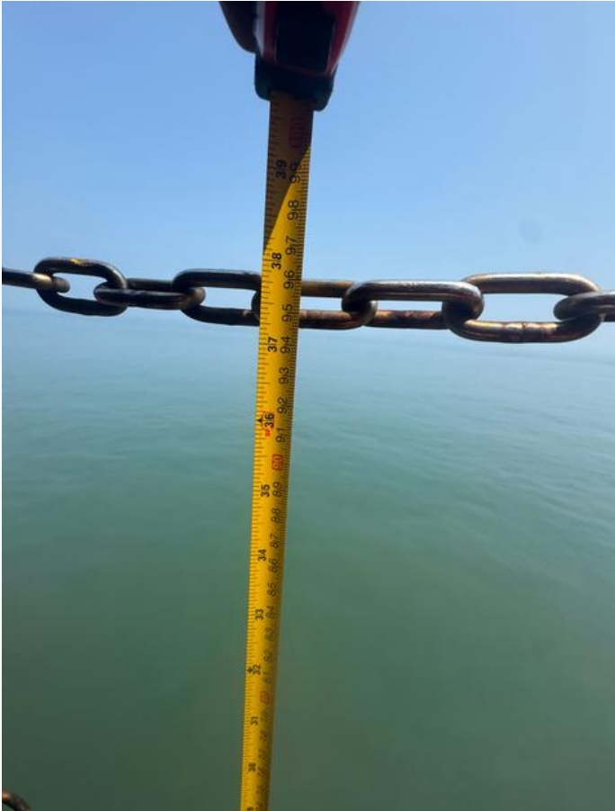
1. The top guard chain should be approximately 1.0 metre above deck level, securely rigged, properly tensioned and maintained in good condition.
