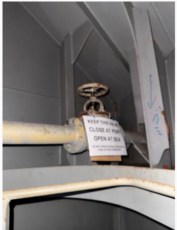
2. During a routine deck inspection, a forward dewatering valve was found in the open position while the vessel was alongside. The operating instruction attached to the valve clearly stated: KEEP THIS VALVE CLOSED AT PORT – OPEN AT SEA
