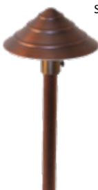
AL20SMAHL12CAR Size: 17.00" x 5.50" dia. Material: Copper Material Options: N/A LED: 3w Omni SS LED (L12) CCT: 3000K Lumens: 300lm ● COP
