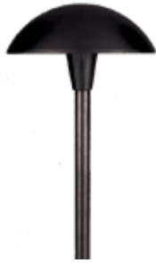
AL12L12BLT Size: 24.00" x 8.00" dia. Material: Aluminum Material Options: Brass LED: 3w Omni SS LED (L12) CCT: 3000K Lumens: 300lm LED Option: LED Panel (LEDP) CCT: 3000K/5200K ● ALUM ● BRS
