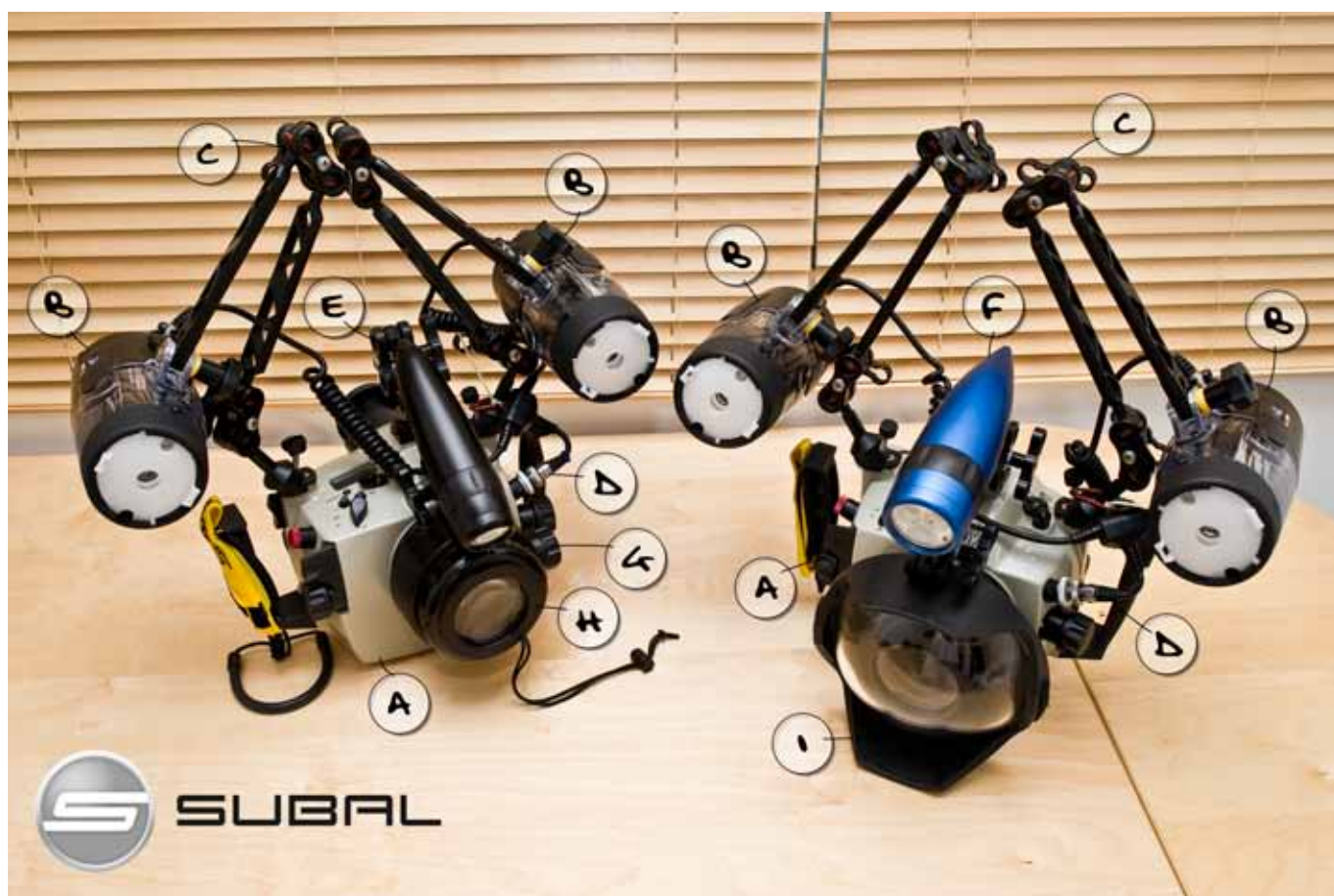
EQUIPMENT KEY BREAKDOWN: a) Subal ND2 Underwater Camera Housing | b) Sea & Sea YS250 PRO Strobes | c) Ultralight Strobe Arm | d) Sea & Sea Nikonos 5 Pin Dual Sync Cord | e) BossK 1x5 LED Underwater Video & Focus | f) BossK 3x5 LED Underwater Video & Focus Light | g) Subal Flat Port | h) Woody's Wet Diopter | i) Subal 8" Dome Port
