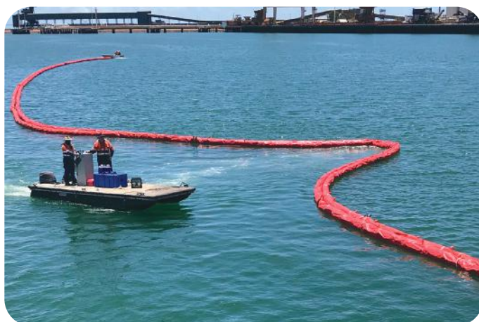
EXPANDI RapidBoom self-inflatable rapid deployment boom
