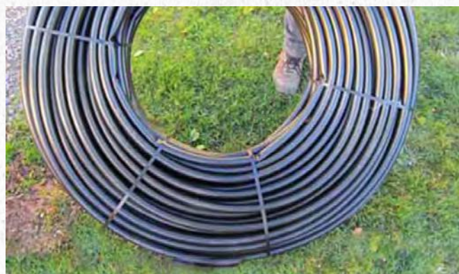
Header/ Main Line Pipe
