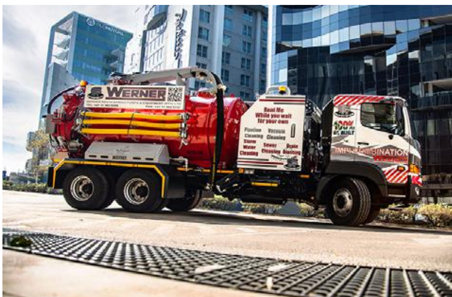
An example of a combination jetting and vacuum truck that was delivered to Walvis Bay
